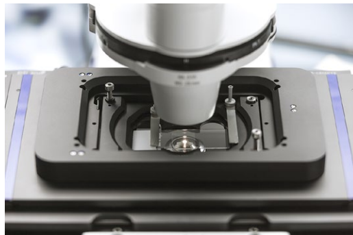
Z piezo stage and a leveling insert guarantee the precision needed for superresolution applications using Airyscan.
