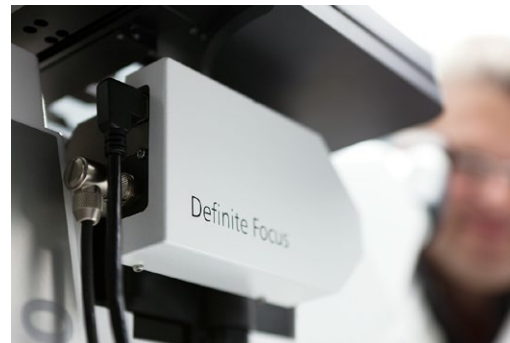
Definite Focus stabilizes the focal position of your sample compensating z-drift. You can now perform long-term experiments that can last for multiple days.
